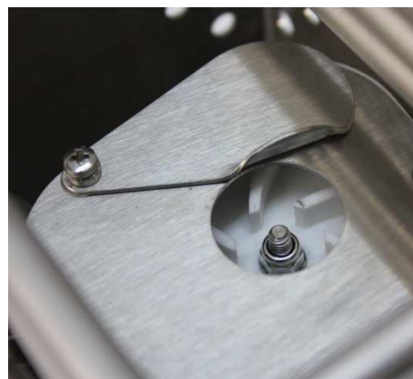
Pump adjusted to maximum flow rate
