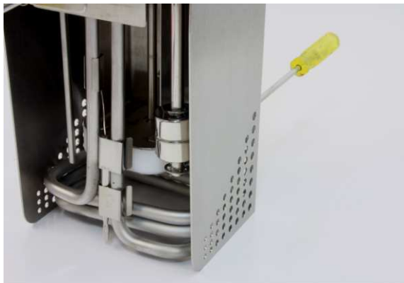
Use a long thin screwdriver to lift the low level float bulb
