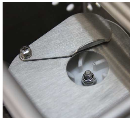
Pump adjusted to maximum flow rate
