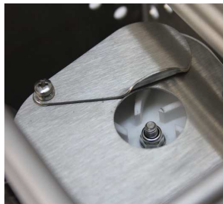
Pump adjusted to maximum flow rate
