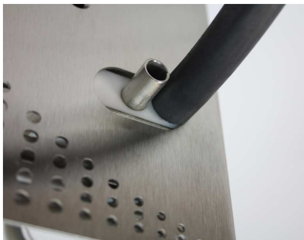
Hose attached for external pump-out
