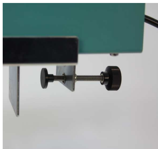
Step 2 – Use the thumb-screw to tighten against the bath
