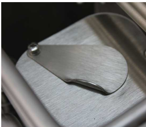
Pump adjusted to minimum flow rate
