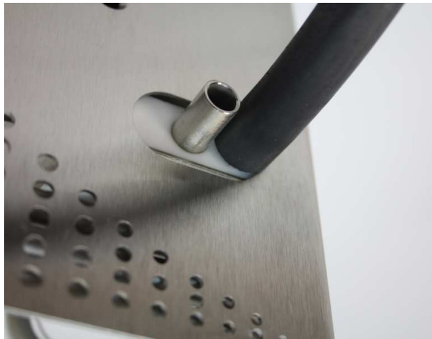
Hose attached for external pump-out
